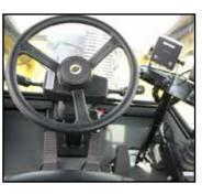
Dashless cab design provides completely unobstructed forward visibility, while the large cab area provides ample leg and elbow room.
