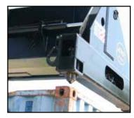
Automatic pendular floating twistlocks with override function; integral carriage with  $^{+/-}30$ " sideshift.
