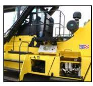
Separate battery cabinet with power disconnect. Separate filter cabinet provides one central location to make for ease of preventative maintenance.
