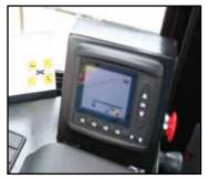
Electronic push-button parking brake control and easily accessible emergency shutdown switch.
