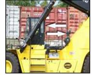
Independently powered traversing cab moves operator forward/ backward for optimal visibility and service access.
