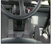
Dual brake pedals - left for brake and declutch, and the right for brake only.
