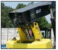
Inclination sensor and optical distance sensor used for locating precise position of container for safety interlocks. Angle and position sensors have no mechanical components for minimal maintenance and improved reliability.
