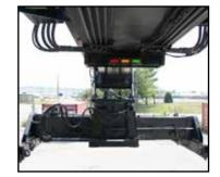
Twistlock engagement indicator lights on boom, as well as inside operator's cab. Interlock safety system ensures proper locking sequence and includes an overload warning alert.
