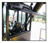
Rear window easily opens for emergency exit. Tinted glass, sliding side windows, push-open rear window and front/rear/overhead wipers provide optimum safety and visibility.
