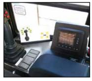
MD3 display features gauge and warning functions, diagnostic capabilities and user interface for making vehicle adjustments.
