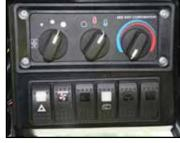
Standard cab heater (air conditioning system is optional). Controls within easy reach of operator's seat.
