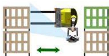
Standing to the side of the stacker eliminates the risk of being trapped or crushed while allowing the Combi-CS to operate in very narrow aisles.
